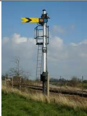
**DISTANT signal:** would be present at the start of the BLOCK SECTION. This should be a fixed signal if there is special caution required, for example a junction within the BLOCK especially on a falling gradient through a tunnel such as we have for Finchley.
