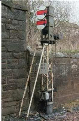
**SHUNT signal:** Primarily this allows a shunting movement across running lines, often against the normal train direction of the line, and permits movement for as far as the line is clear and no further. They are generally discs but not always ground level as this image shows; visibility for the train crew is important.
