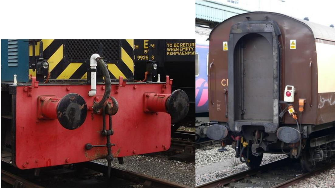
Class 04 showing screw coupling and vacuum pipe, Mark 1 coach showing buckeye coupling in the 'rest' position.
